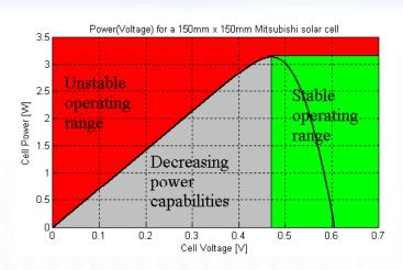
In the stable region if the output power is less than the input power, the remainder shows itself in an increased DC-bus voltage which causes a subsequent decrease in power input, creating an ultimately stable system without additional control mechanisms.
